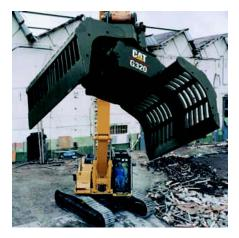
**Lowering Control Devices.** Lowering control devices are installed on all boom and stick cylinders.
