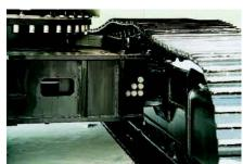
**Optional Hydraulic Adjustable Undercarriage.** The optional hydraulic adjustable undercarriage increases the stability by lowering the center of gravity of the machine, resulting in the usage of a bigger tool. The non-bolt joint allows changing from shipping to working width or reverse in less than a minute.
