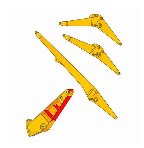
**Demolition Sticks.** Purpose built demolition sticks have additional internal reinforcements, heavier plates, through hardened bores and a bottom wear plate and match the short boom nose.
