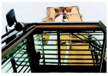
**Falling Object Guard.** Falling object guard on the top and front is standard. Crossbars of top guard are angled in line with sight for enhanced visibility to the tool.
